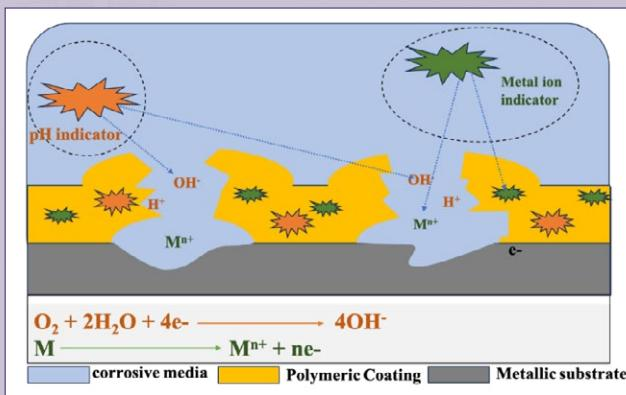
**Figure 1:** Scheme of mechanisms of corrosion detection, detecting local pH, Metal ions, or mechanical damage caused by corrosive media.
