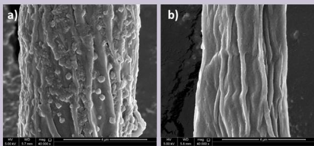
**Figure 2:** a) Representative scanning electron microscope image of the raw and b) alkali-treated *P. undulata* fibers, showing the loss of hemicellulose, lignin, and bioactive extractives from the raw fibers after alkali treatment.
